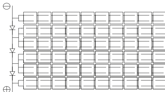
Figure 7: Electrical circuitry of cells and bypass diodes
